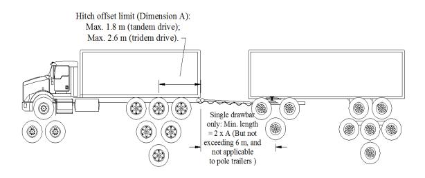
In 2011, British Columbia agreed with government in Alberta and Saskatchewan to increase the maximum hitch offset limit for a tridem drive truck by 0.1 m, i.e., from a maximum 2.5 meters to 2.6 meters, to ensure consistency in cross border travel.
