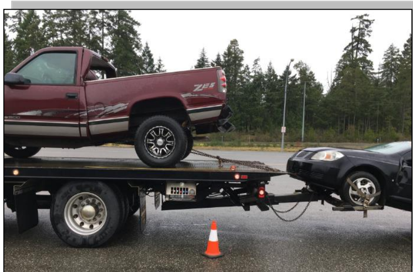
Figure 1: Flatbed tow truck with wheel lift towing a motor vehicle
